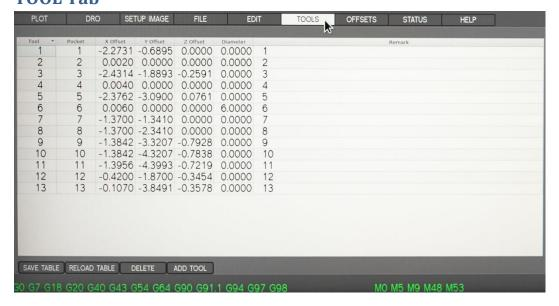
The Tool tab displays the tool table. Tool offsets allow the operator to use tools of different lengths in different tool locations while still programming with respect to the workpiece. You can switch tools quickly, without setting up the mill every time a tool is mounted. The current tool's offset values are in the DRO tab (TLO) for you to see anytime.
