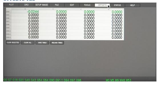
The Offsets Table displays the current offsets for the active work coordinates (G54). The current G5X values are in the DRO tab for you to see at anytime. To alter a value in the table, mouse-click twice on the field that you'd like to edit. When you finish entering the desired new value, click Enter key on the keyboard to accept the value.
