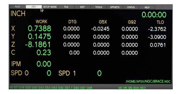
This tab shows detailed information in a dashboard style. For example, you can see the current unit inch or mm. The work coordinates are in the first column. The active G coordinates are also on this tab. The current IPM and RPM values are in the lower-left corner. The active file location is listed in the lower right corner. Finally, the duration of the g-code is placed in the top right corner.
