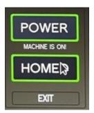
When using the EXIT button, the machine will save the G54 coordinates homing positions based on your workpiece. When you are done using the machine, you can **unplug the power cord from the wall outlet** if you do not need to keep the homing coordinates.
